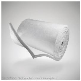
ITM-Fibermax® are high-temperature, lightweight and flexible products made of polycrystalline mullite/alumina wool (PCW) that can be exposed to temperatures up to 1.600 °C.
